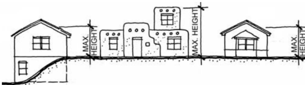
Figure 1. Illustration of Building Height.
